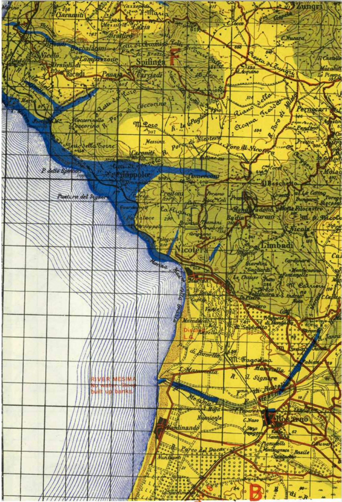
Plate 35. GSGS 4164. Italy. 1 : 100,000. Sheets 245 & 246 with "Going" overprint, based on air photo information. Fair ■ Bad ■ Impassable. ■
